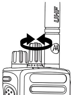
Once the required zone is set (if you have multiple zones in your radio), turn the programmed Channel Selector Knob to select the call type.
