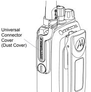
Place the universal connector cover loop over the attached antenna. Slide it all the way down to the base of the antenna.
