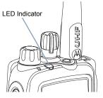
**NOTE:** The LED lights up solid green while the radio is transmitting and blinks green rapidly when the radio is receiving a privacy-enabled call.
