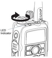
**NOTE:** The Home screen does not light up during a power up if the LED indicator is disabled (see *Turning the LED Indicator On or Off* on page 83).
