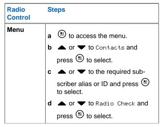
The display shows the Target Alias, indicating the request is in progress. The LED lights up solid green.
