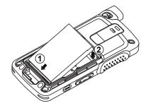
**2** Push the top of the battery down until the latch snaps into place.
