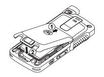
3 Slide battery latch into lock position.
