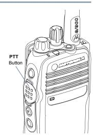
While a call is not in progress, the PTT button is used to make a new call (see Making a Radio Call on page 14).
