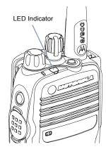
**Blinking yellow** – Radio is scanning for activity or receiving a Call Alert.
