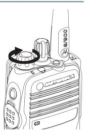
If your radio does not power up, check your battery. Make sure that it is charged and properly attached. If your radio still does not power up, contact your dealer or system administrator.
