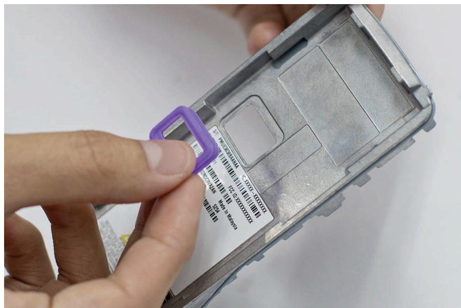
Figure 24: Battery contact seal removal
