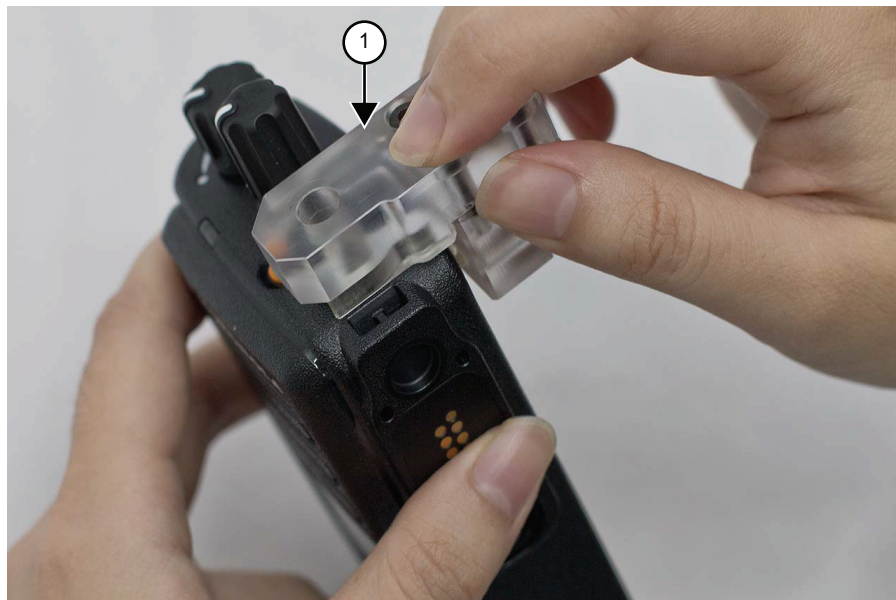
Figure 10: RF Adaptor insertion
