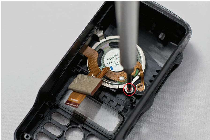
Figure 33: Speaker retainer screw removal
