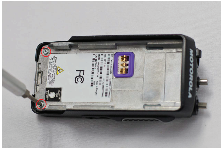
Figure 17: Front Kit-Back Kit Screw removal
