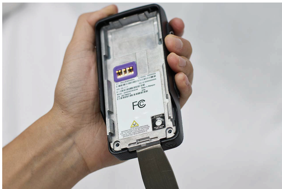
Figure 18: Back Kit disassembly
