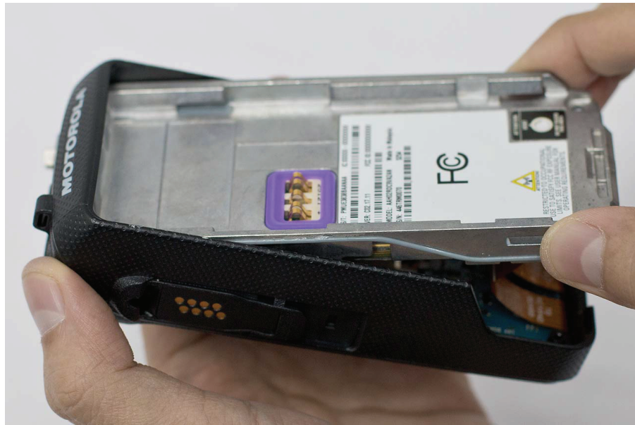
Figure 19: Back Kit removal
