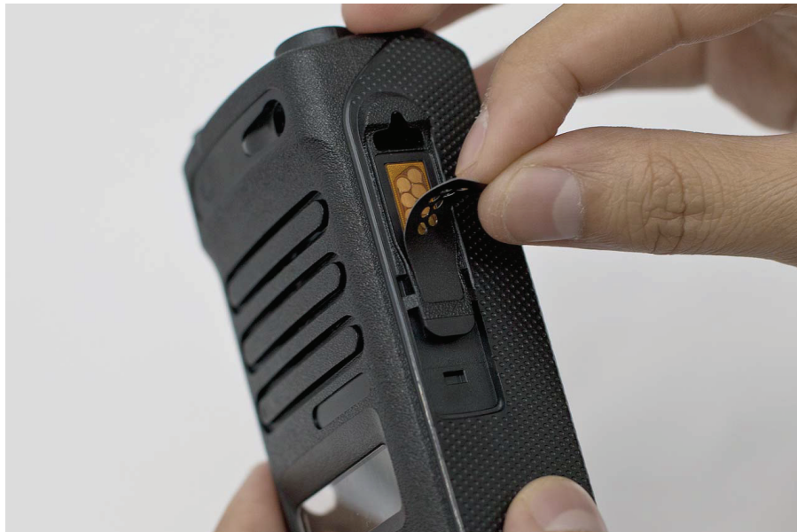
Figure 31: UC escutcheon removal
