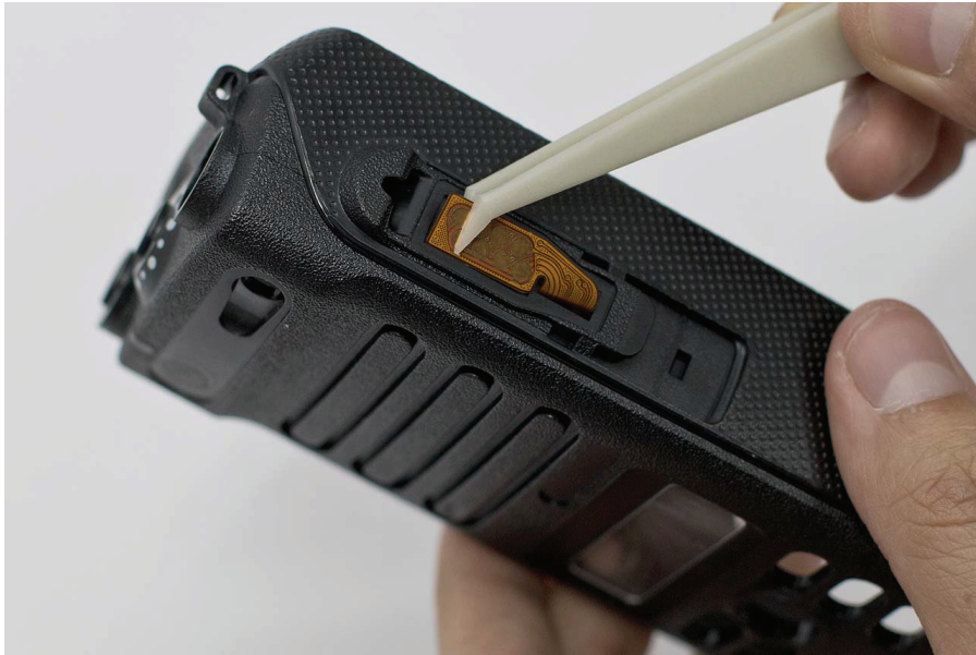
Figure 32: UC-audio flex removal
