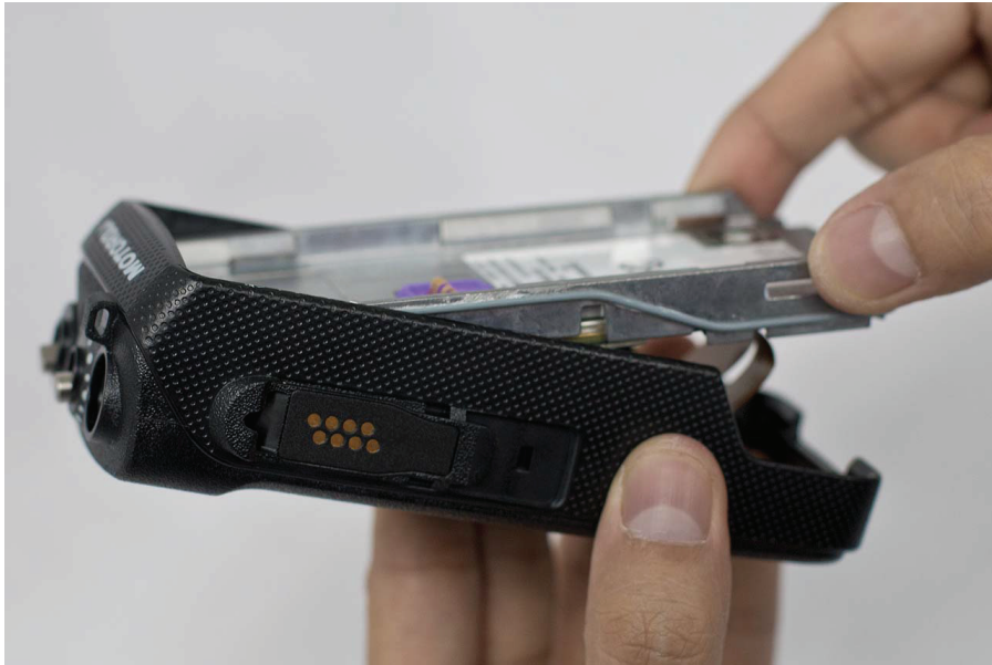
Figure 54: Front kit reassembly
