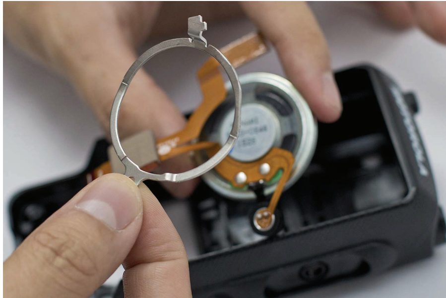
Figure 34: Speaker retainer removal
