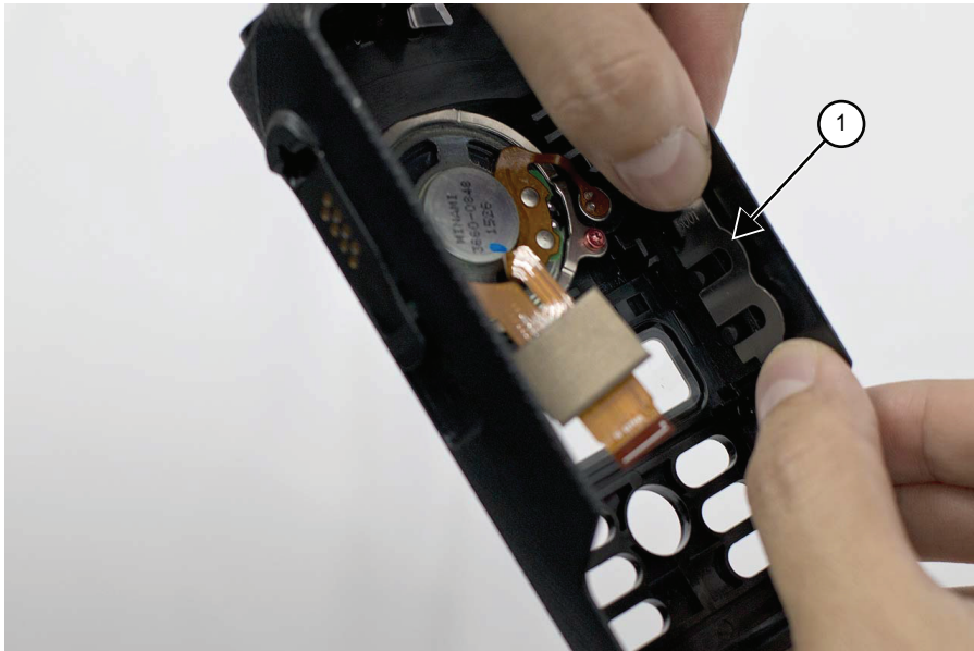
Figure 29: PTT retainer removal
