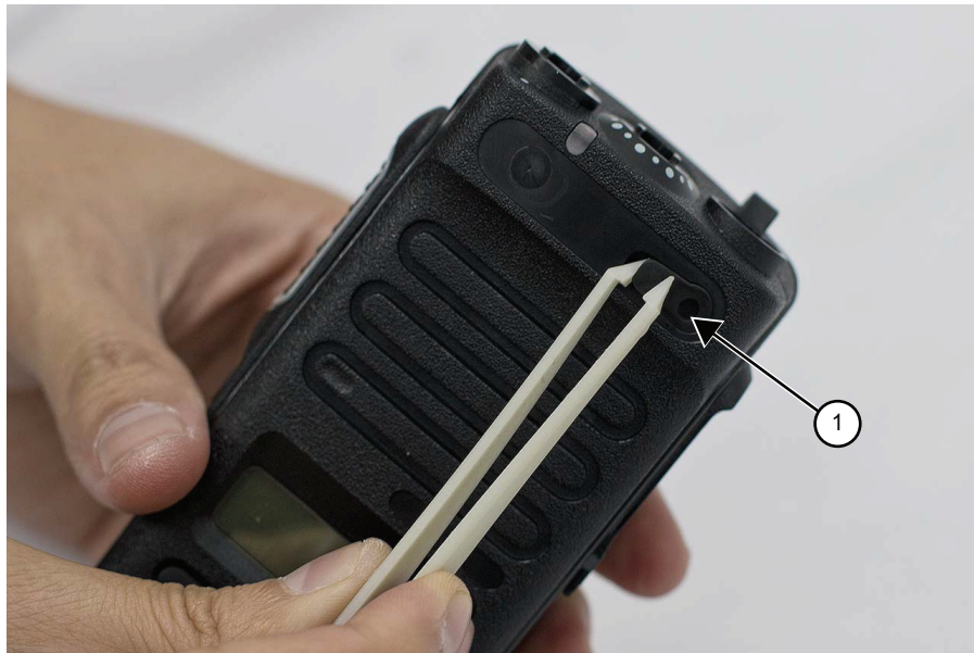
Figure 9: RF Plug disassembly
