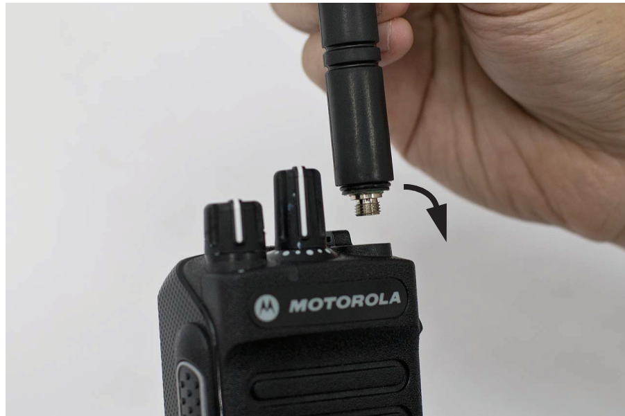
Figure 56: Attaching the antenna
