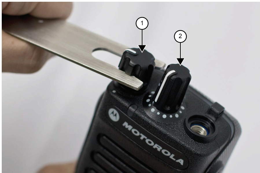
Figure 16: Volume and Channel Knob removal.
