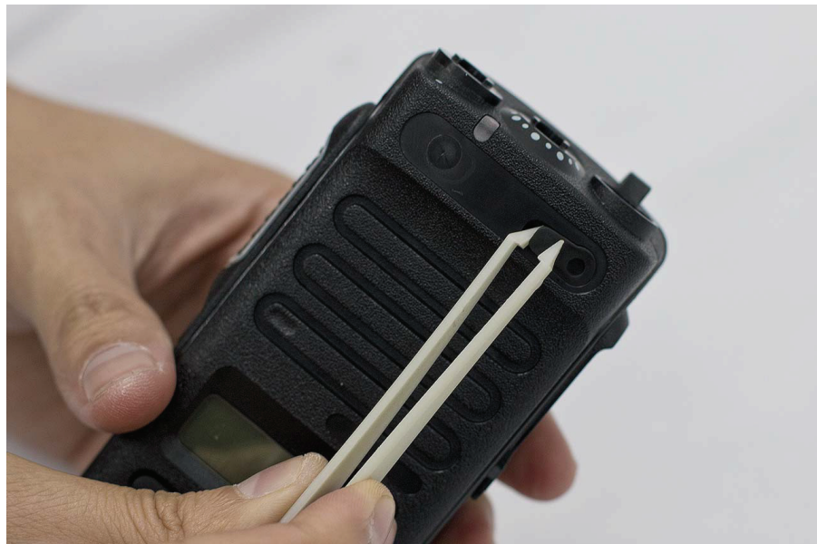
Figure 57: RF Plug reassembly
