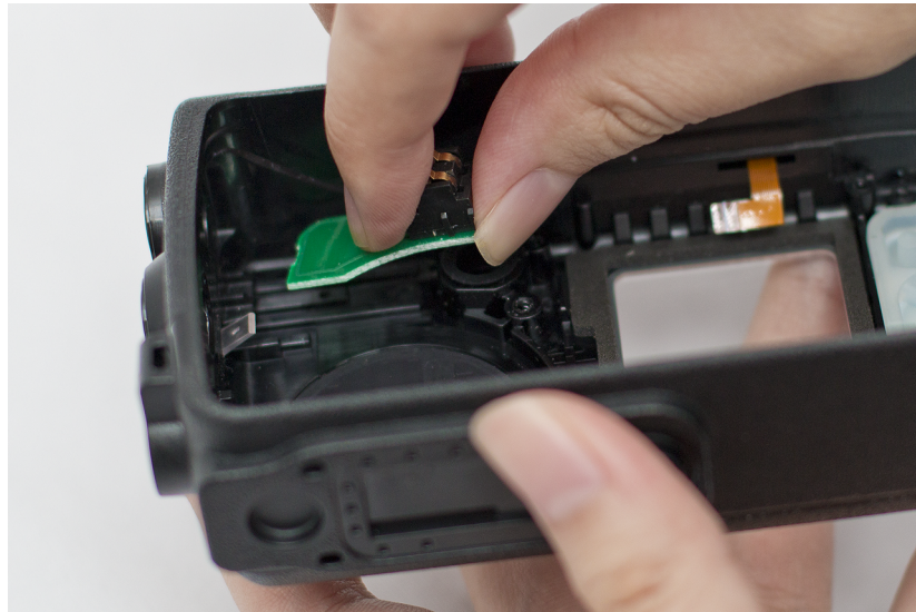
Figure 42: Bluetooth GPS Antenna Removal
