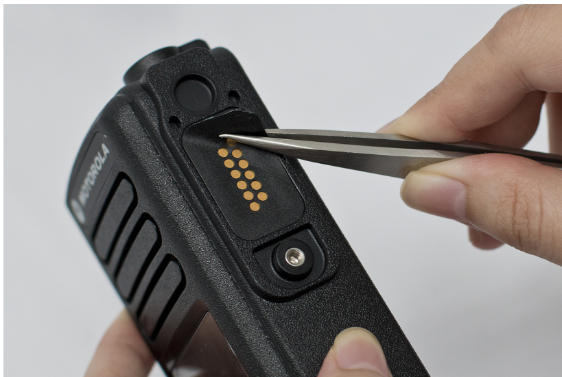
Figure 46: UC Escutcheon Replacement
