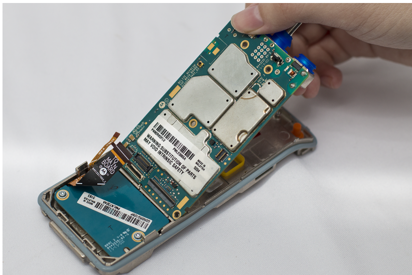
Figure 25: Main Board Removal
