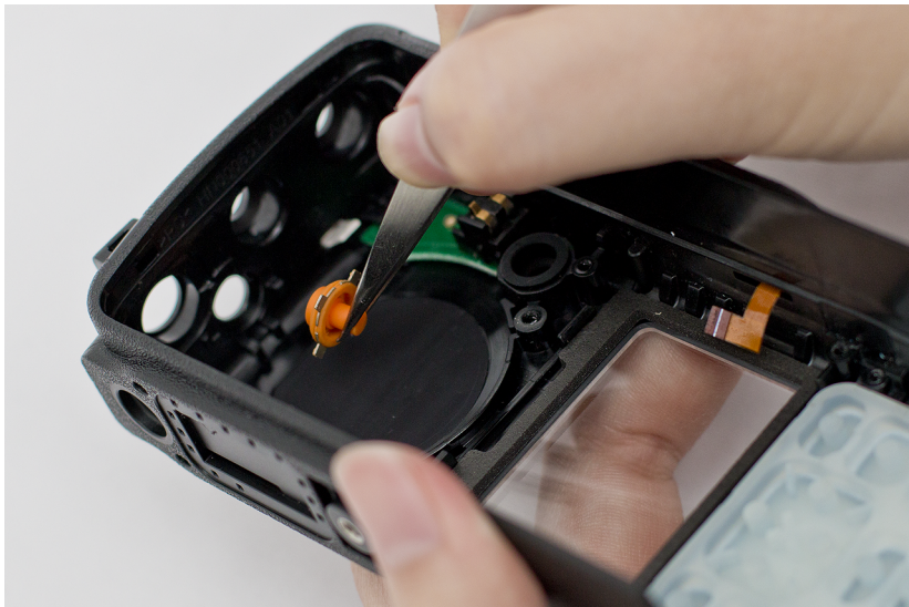
Figure 41: Emergency Button Removal
