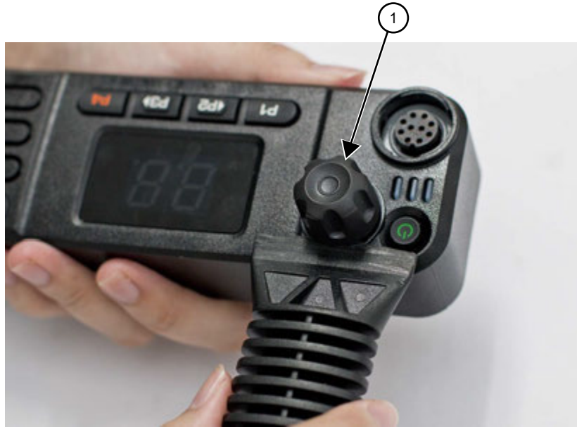
Figure 47: Volume/Channel Knob Removal
