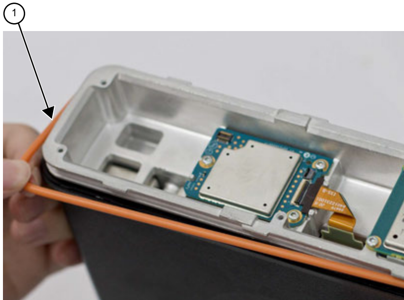
Figure 103: Assemble O-ring to Chassis (Image May Not Match Exact Product)
