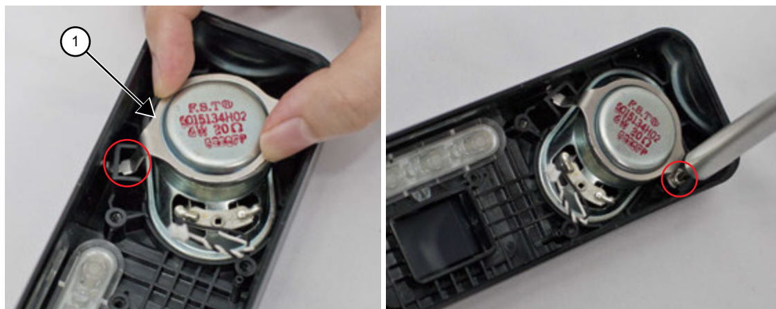
Figure 73: Speaker Retainer Assembly
