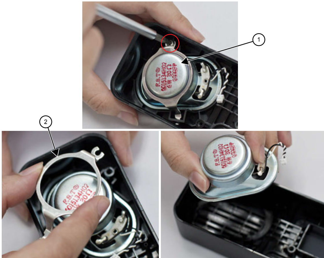
Figure 53: Speaker Removal (Optional)
