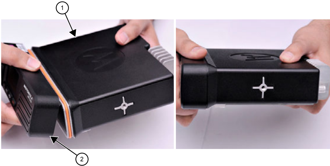
Figure 106: Assemble Control Head to Radio Chassis
