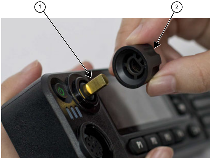
Figure 67: Volume/Channel Knob Assembly
