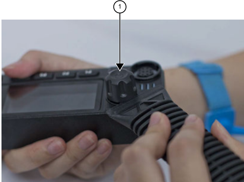
Figure 33: Volume/Channel Knob Removal
