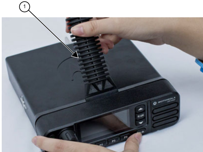
Figure 10: Typical Control Head Removal
