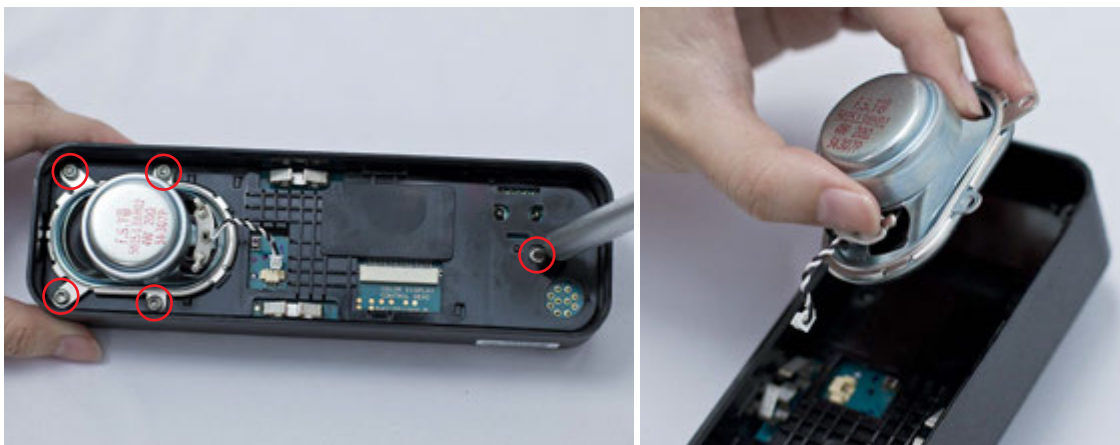
Figure 34: Control Head Screws and Speaker Removal
