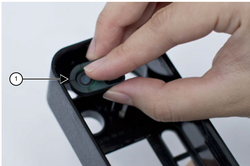
Figure 68: Power Button Placement
