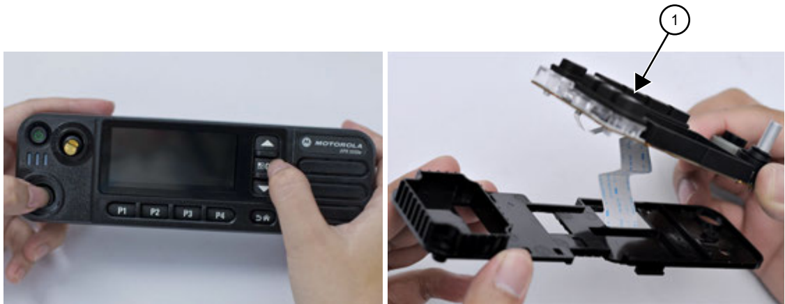
Figure 36: Control Head Board Removal
