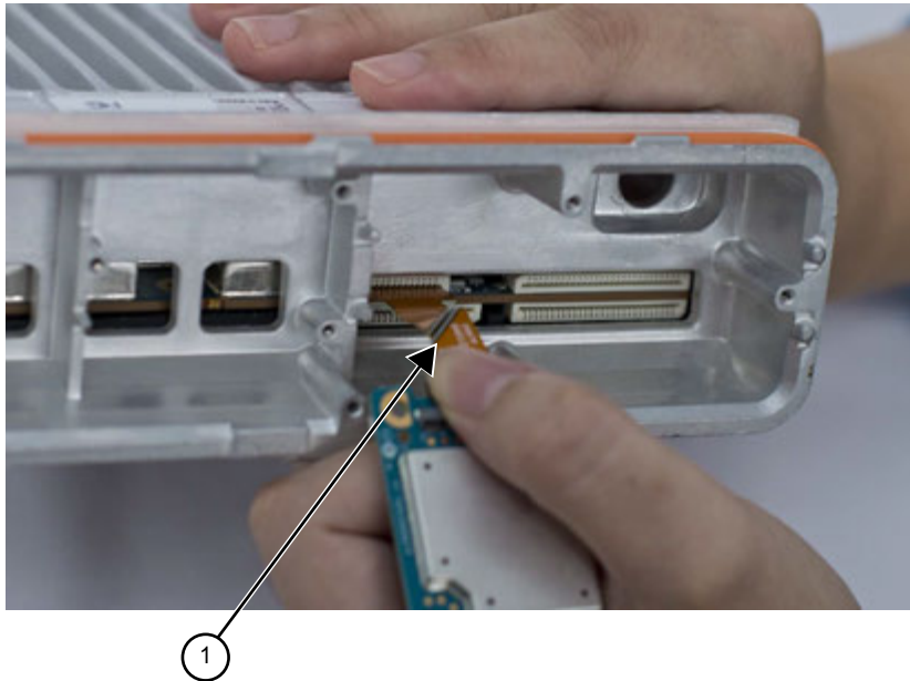
Figure 21: Option Board Flex Removal (Image May Not Match Exact Product)
