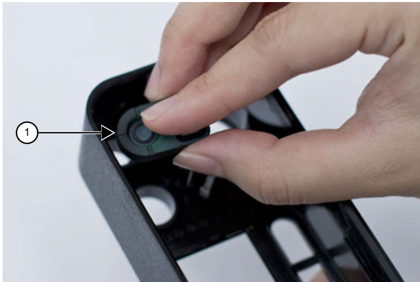
Figure 55: Power Button Placement
