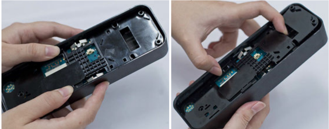
Figure 35: PCB Retainer Removal
