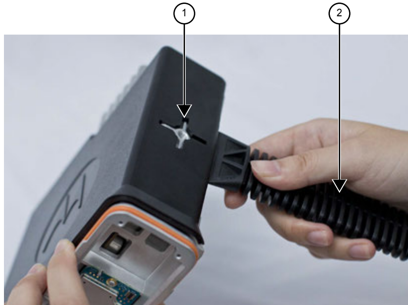
Figure 13: Dismantling Top Cover (Image May Not Match Exact Product)
