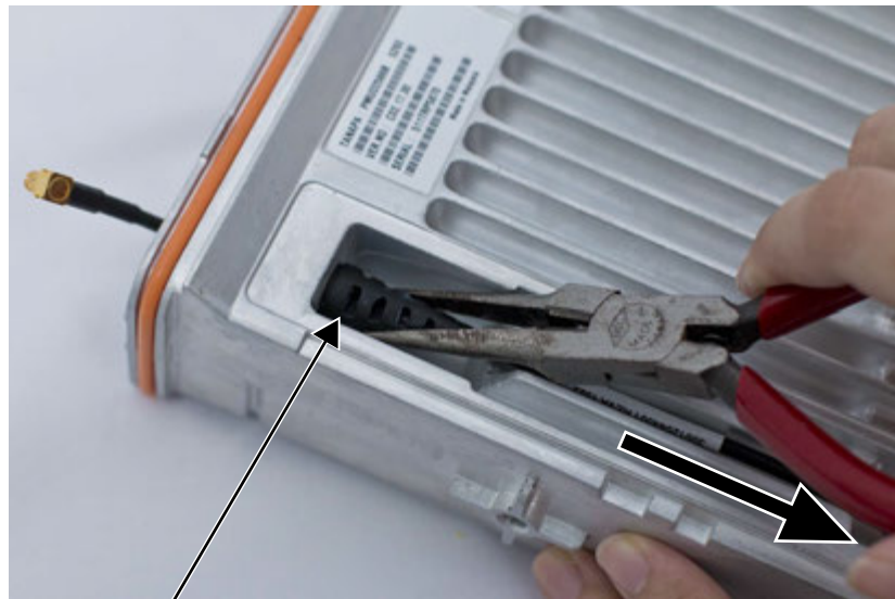
Figure 19: GNSS Cable Removal
