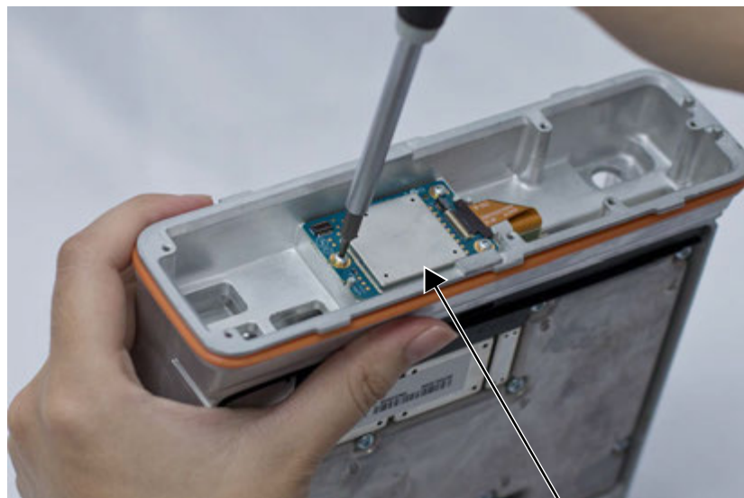
Figure 20: Option Board Removal (Image May Not Match Exact Product)
