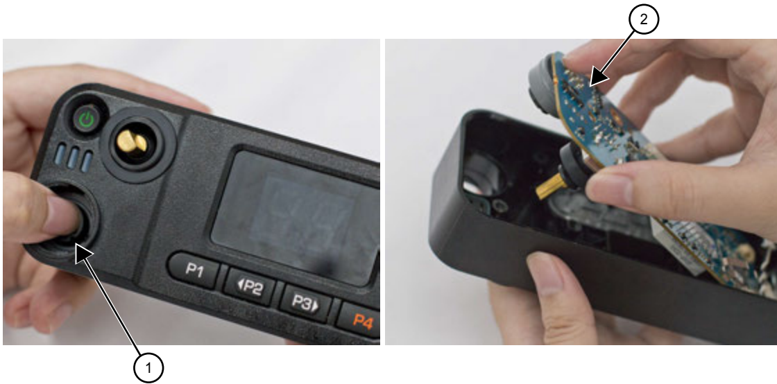
Figure 49: Control Head Board Removal
