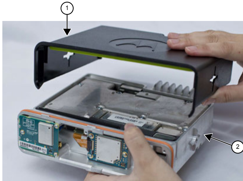
Figure 14: Top Cover Removal
