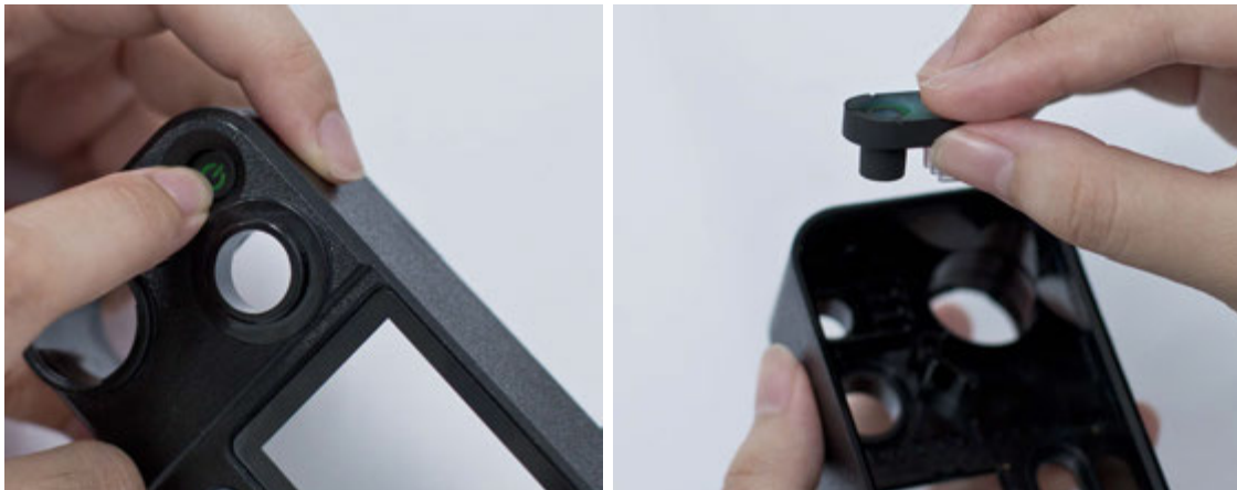
Figure 50: Power Button Removal
