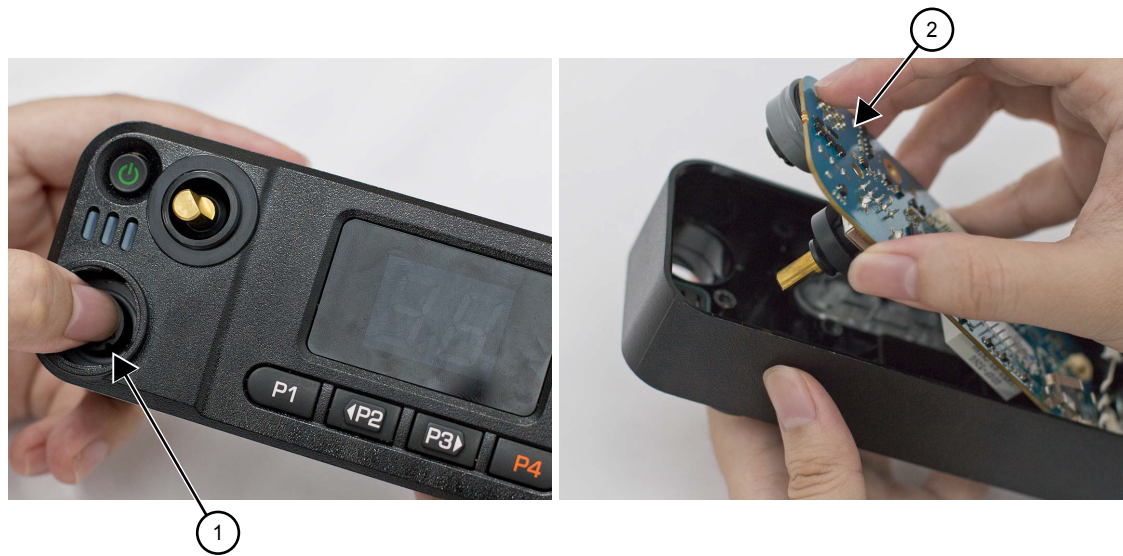
Figure 49: Control Head Board Removal
