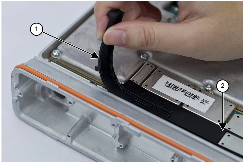
Figure 90: Acoustic Plug Installation
