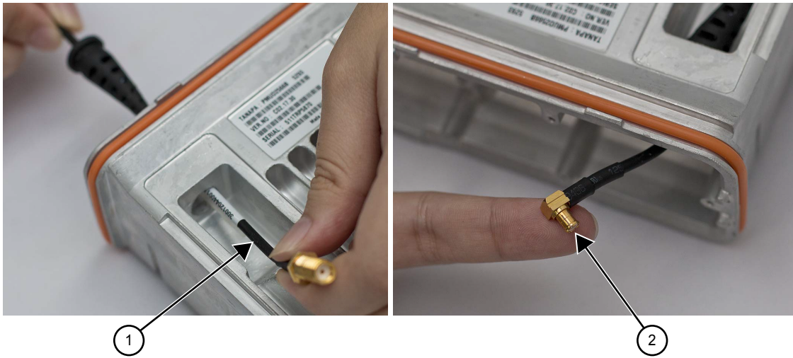
Figure 93: GNSS Cable Installation
