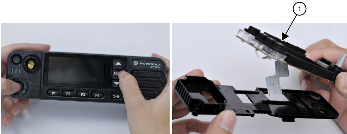
Figure 36: Control Head Board Removal
