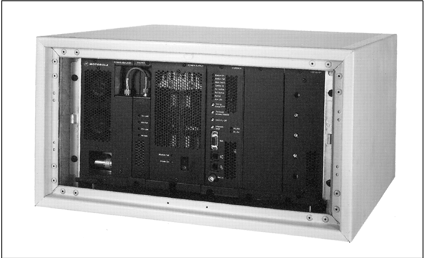
Figure 1. Quantar Station in 12" Cabinet (UHF Shown)
