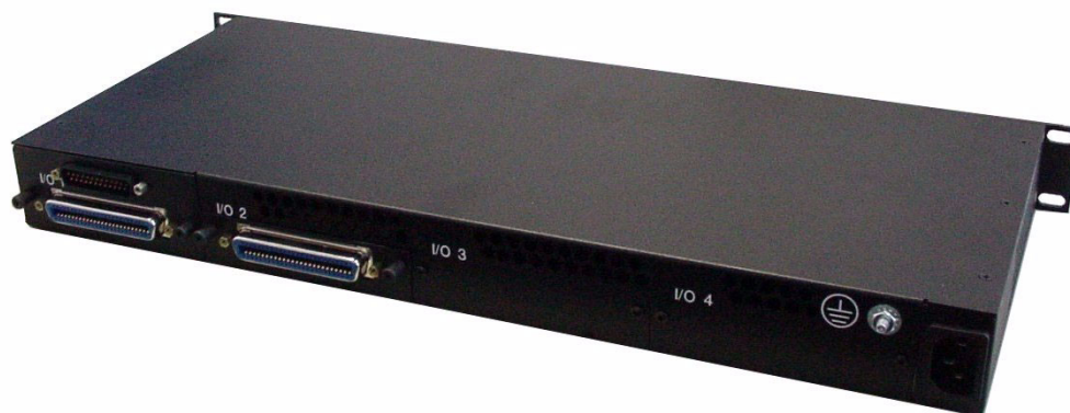
FIGURE 5-3 I/O SHELF (BACK VIEW) WITH TWO I/O MODULES
