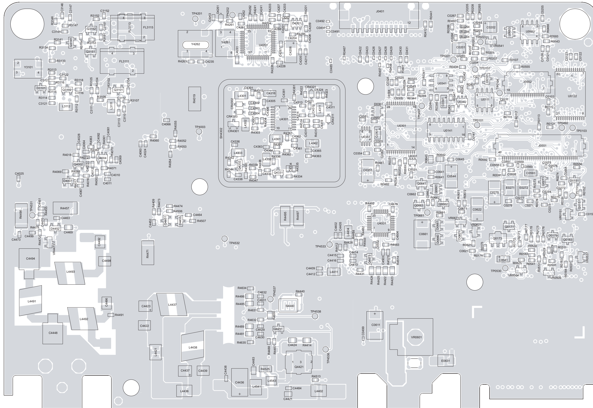
UHF Band 1 (403–470 MHz) 25–40 W LDMOS PCB 8486127Z01 Bottom Side
