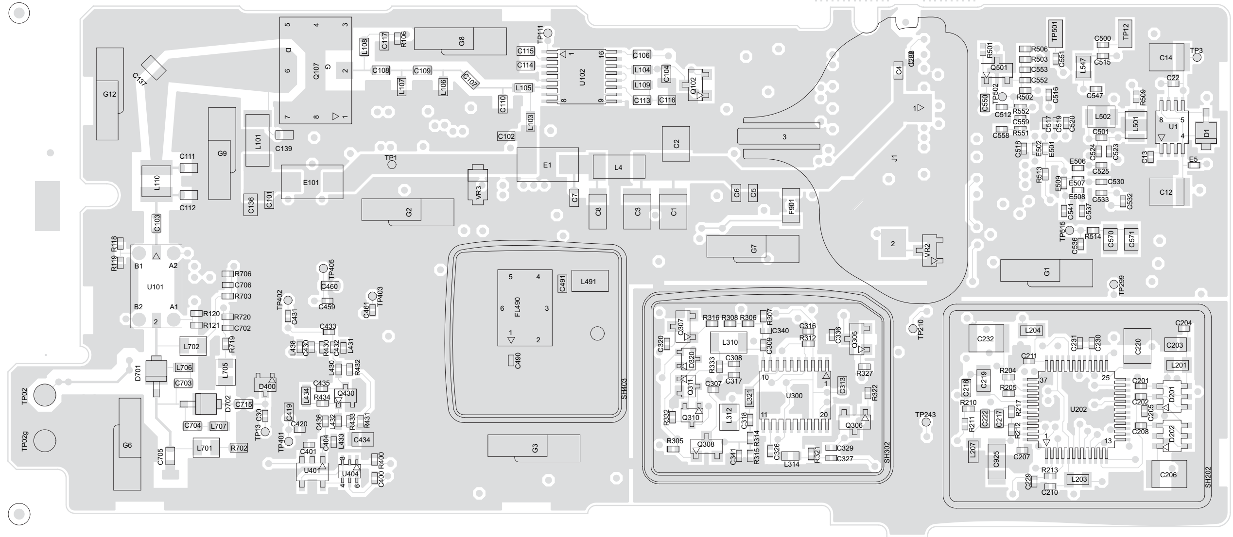
Figure 8-48. NLE4278D UHF Range 1 Transceiver (RF) Board Layout—Side 2
