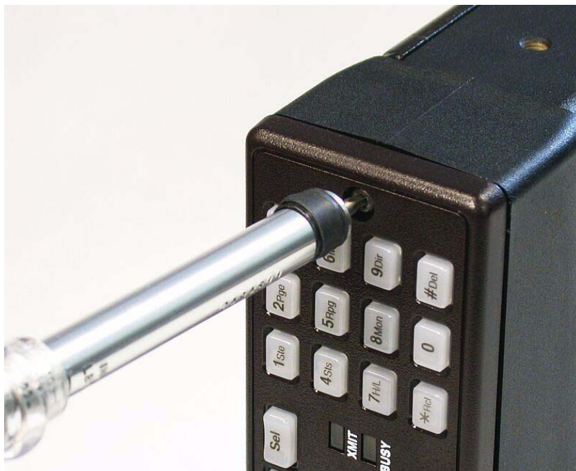
Figure 8-37. Installing the Control-Head Screws
