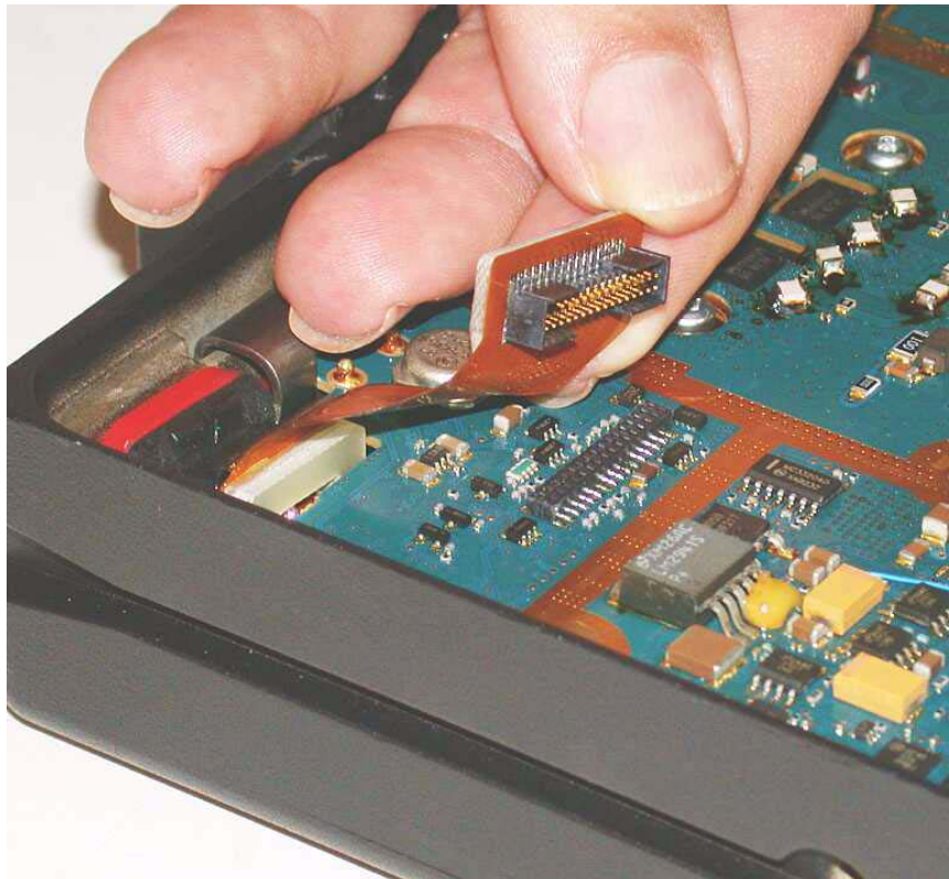
Figure 8-14. Removing the J2 Rear Accessory Flex from the Main Board
