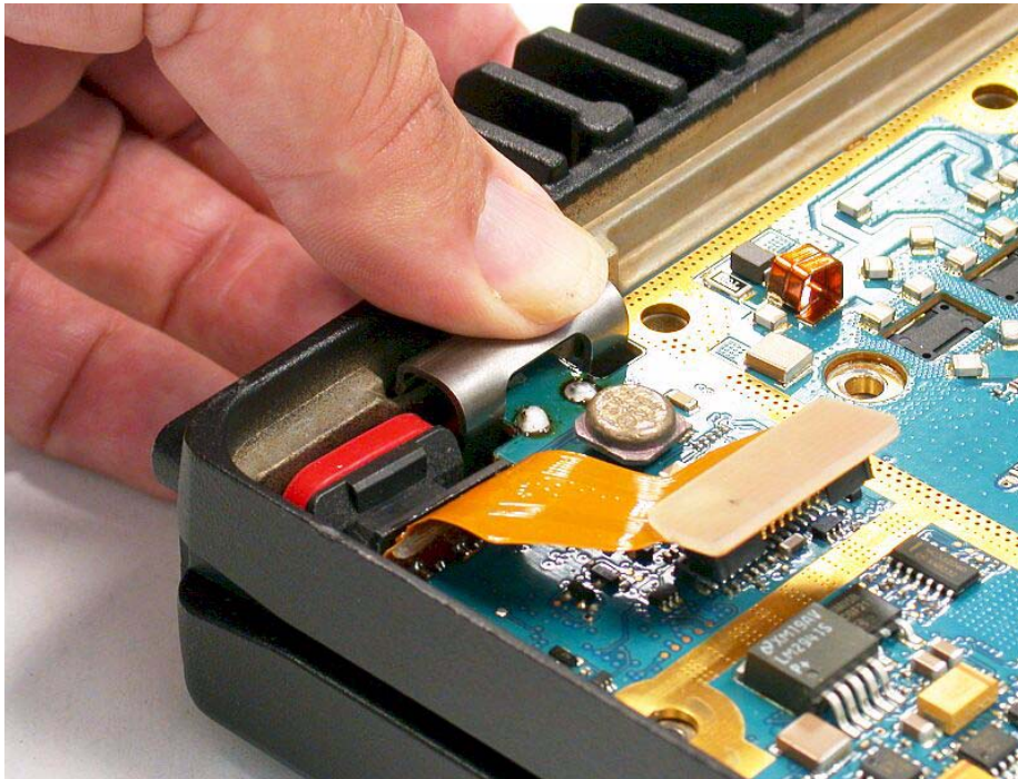
Figure 8-24. Inserting the RF/DC Retention Clip (DC Side)
