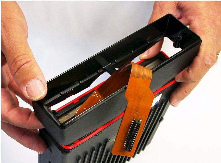
Figure 8-34. Installing the Headbridge on the Transceiver
