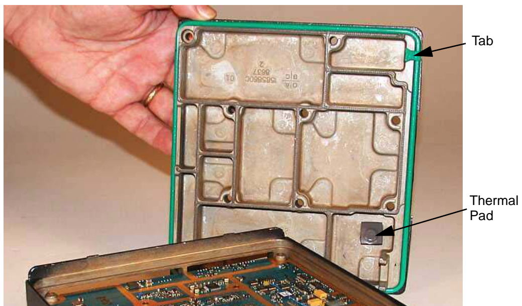
Figure 8-28. Inspecting the Thermal Pad and Installing the Cover Main Seal
