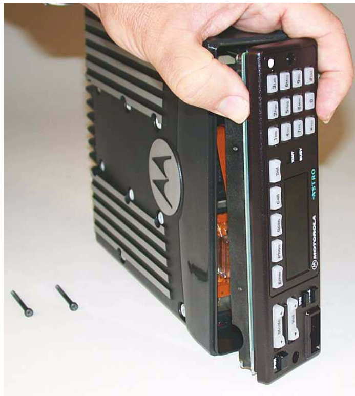
Figure 8-4. Removing the Control Head
