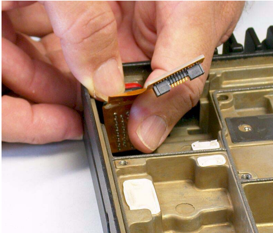
Figure 8-22. Inserting the J2 Rear Accessory Connector
