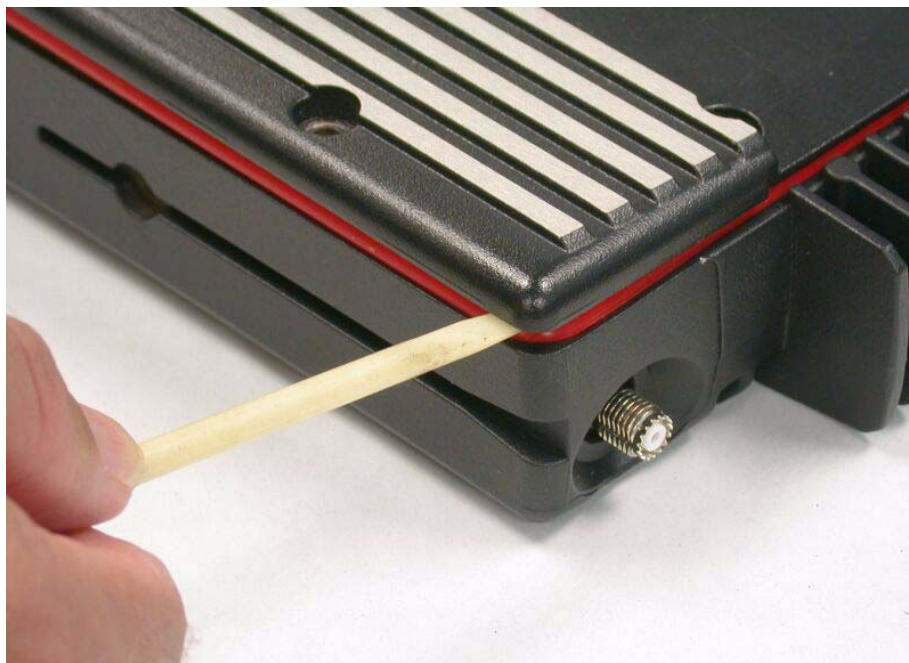
Figure 8-12. Lifting the Top Cover
