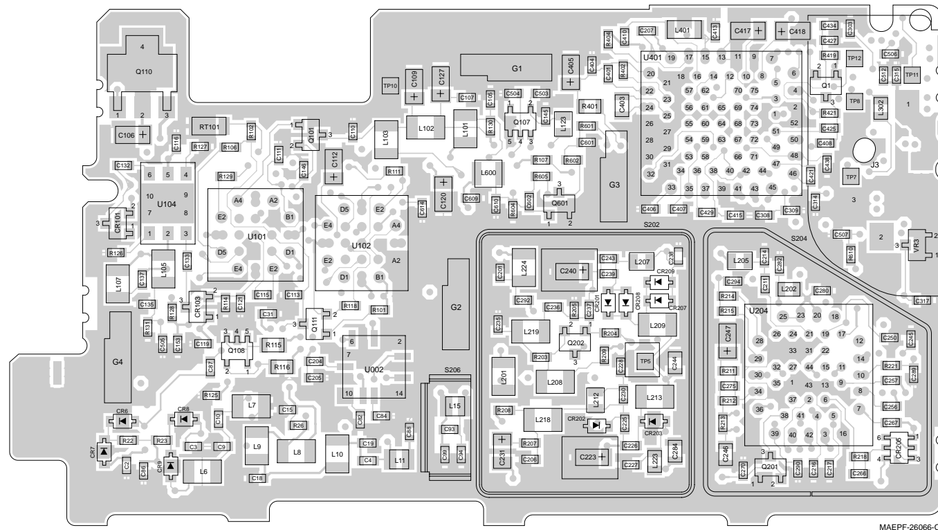
NLE4250B UHF Range 2 RF Board Component Location Detail and Parts List
