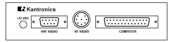
CAUTION: Make sure the power of the transceivers, computer and KAM is OFF before connecting any cables.
