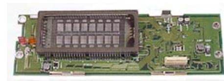
B19/CMC-638C Control Panel Board (For Control Units)
